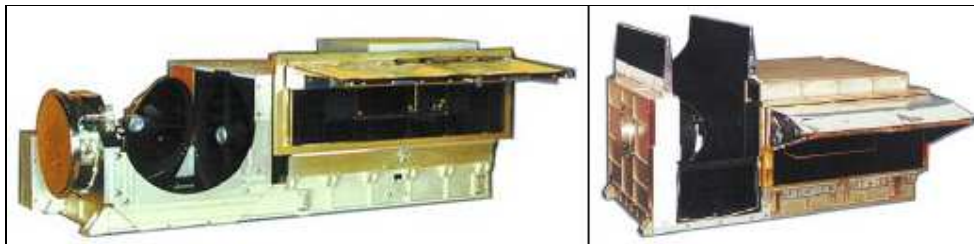
Figure 6. 44 AVHRR and HRIRS Instruments by NOAA 2009
