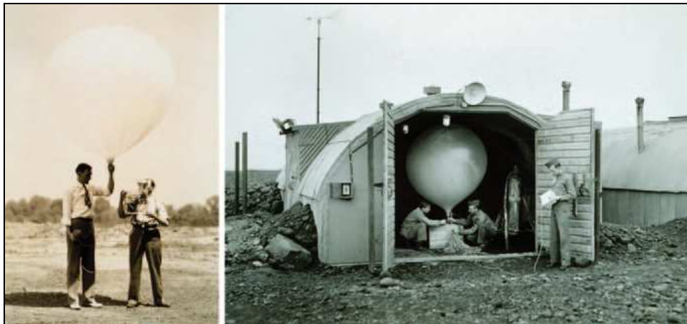
Figure 6. 4 Early Launch of Radiosondes and Preparing Hydrogen-filled Balloon in the Hangar by Tan 2014
