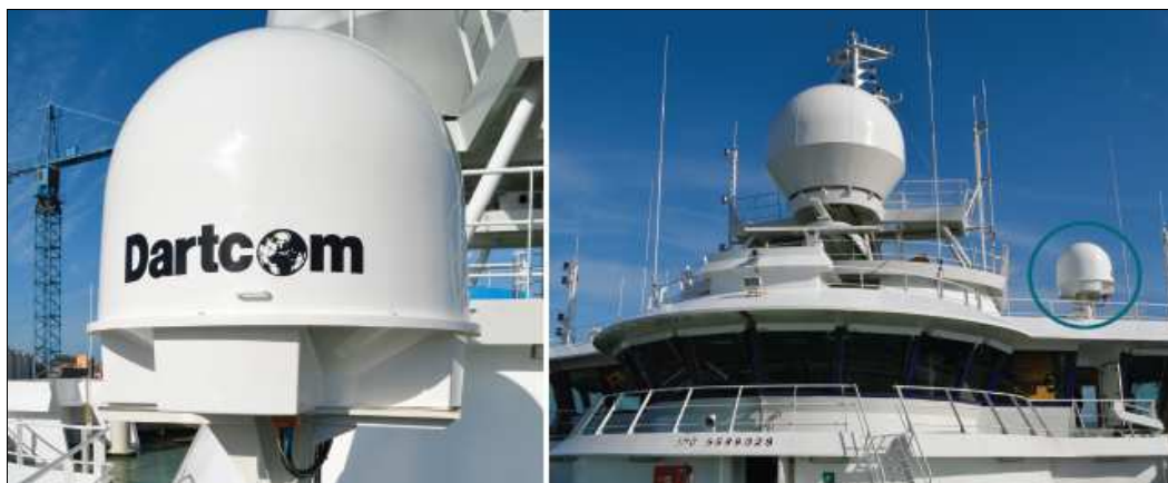
Figure 8. 38 Dartcom 1.3m Active-Stabilized Marine Antenna by SeaSpace 2011
