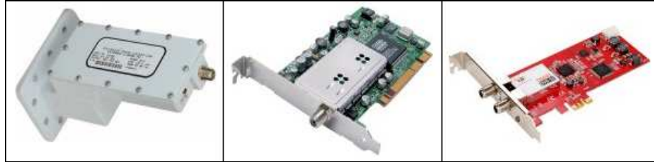
Figure 8. 11 DVB-S2 LNB and PC Receiving Cards by Dartcom 2015
